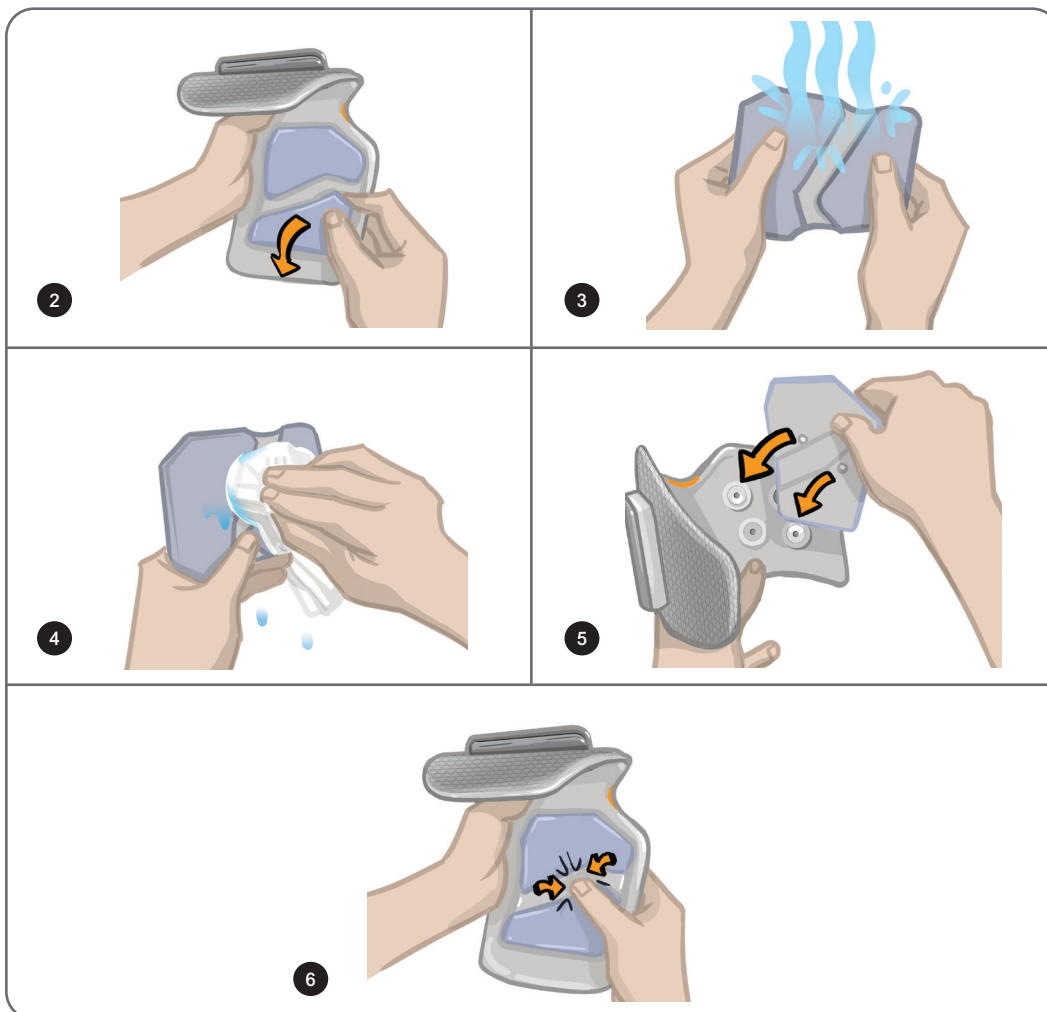
Figure 11-3: Replacing the Quick Fit Electrode
