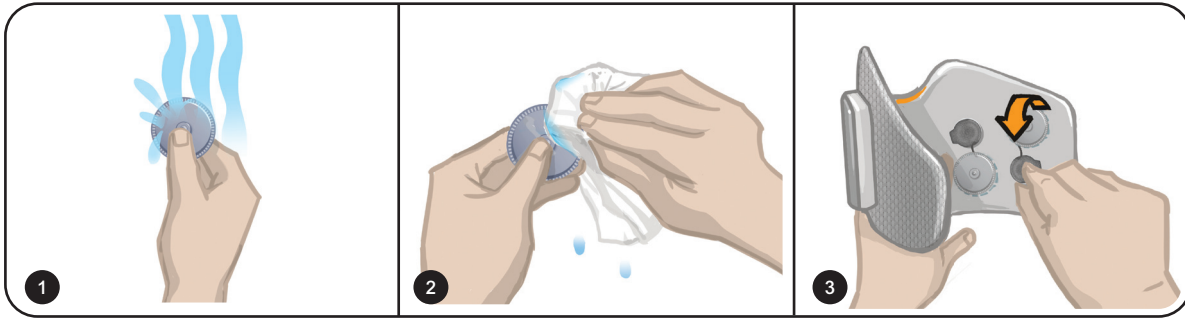
Figure 8-11: Fitting the Round Cloth Electrode
