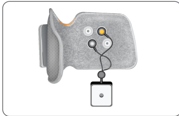
Figure 13-1: Tester Connected to Lower Leg Cuff
