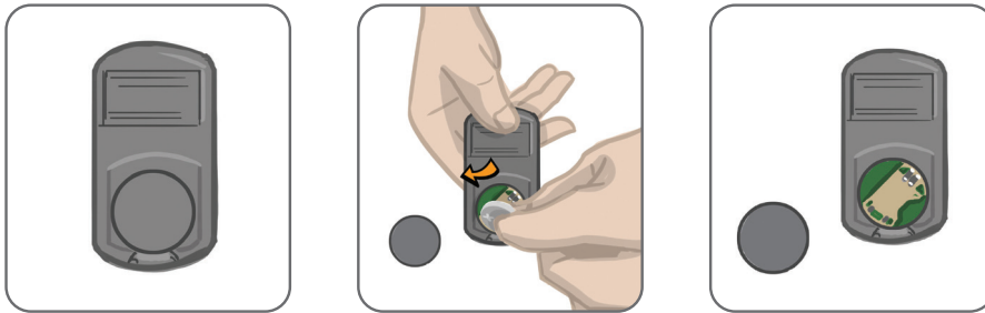
Figure 8-2: Replacing the Control Unit Battery
