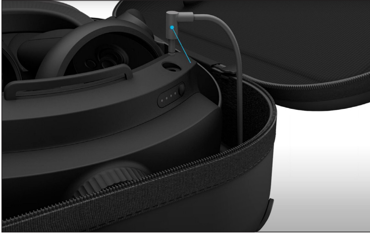
Figure 14-15 Connect the Charge Cable to Back of Headset
