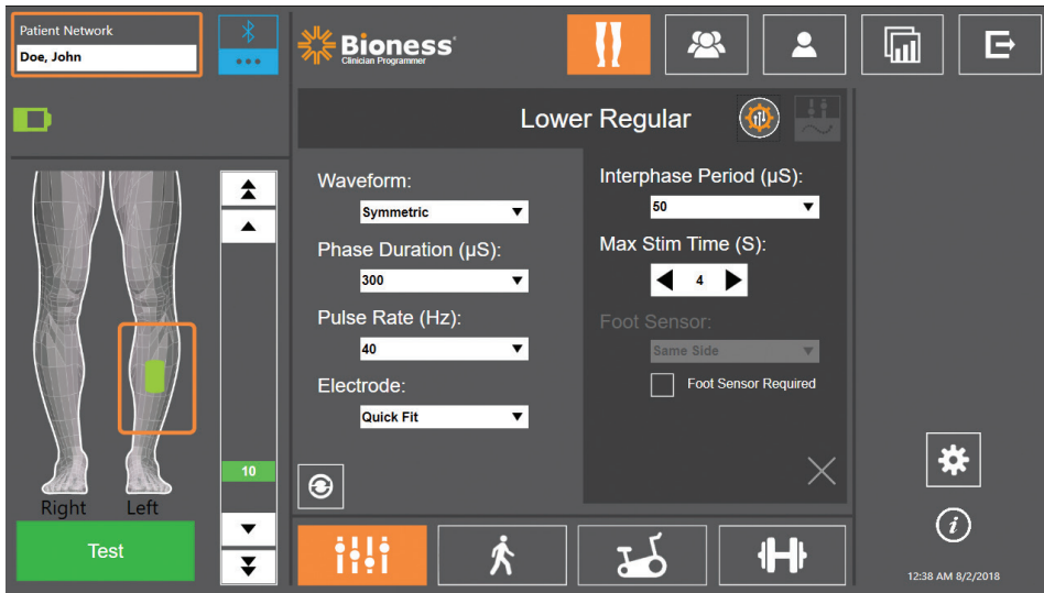
Figure 9-4: Programming Stimulation, Parameter Screen with Advanced Settings Window
