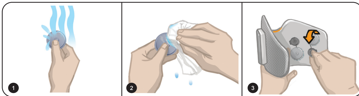
Figure 8-11: Fitting the Round Cloth Electrode
