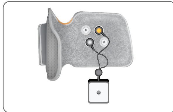
Figure 13-1: Tester Connected to Lower Leg Cuff
