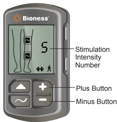
Figure 4-9: Adjusting Stimulation Intensity
