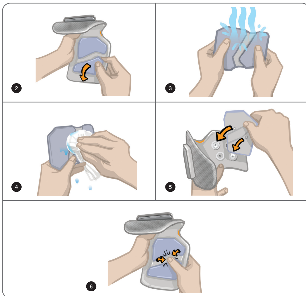
Figure 11-3: Replacing the Quick Fit Electrode
