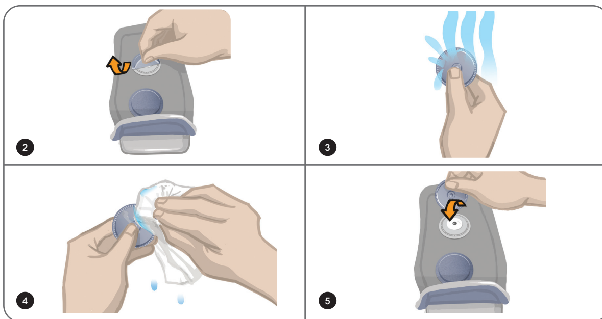
Figure 8-9: Fitting the Small Round Cloth Electrodes
