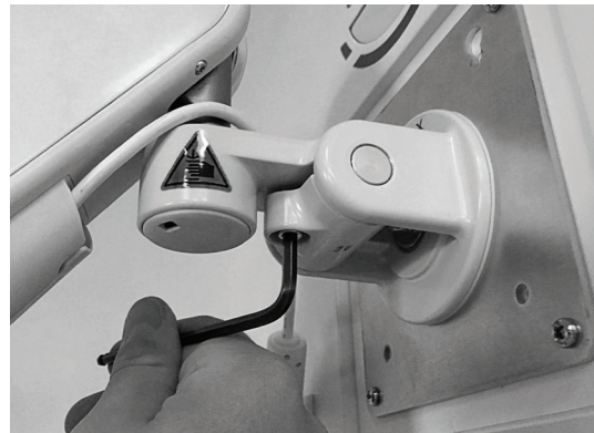
Figure 7: Tilting Tension Adjustment
