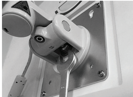
Figure 6: Rotational Tension Adjustment
