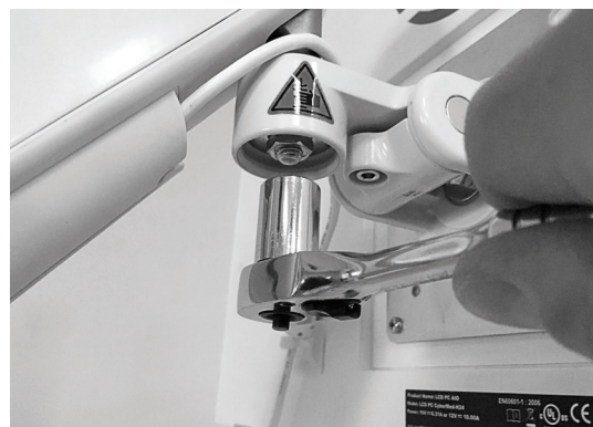
Figure 8: Left/Right Rotational Adjustment
