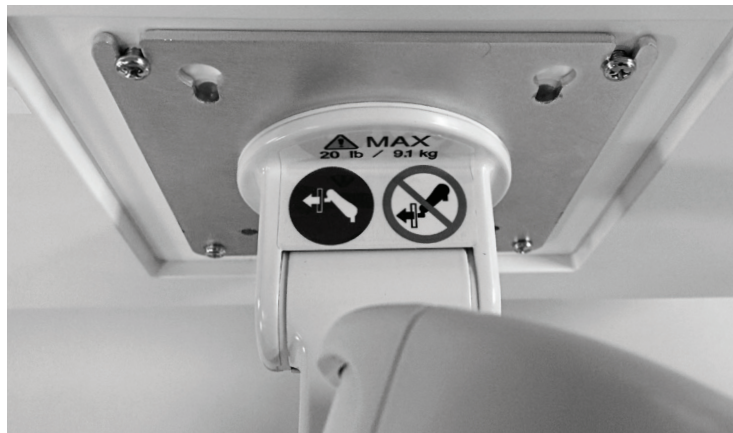
Figure 5: Installed Touchscreen PC on VESA Mount
