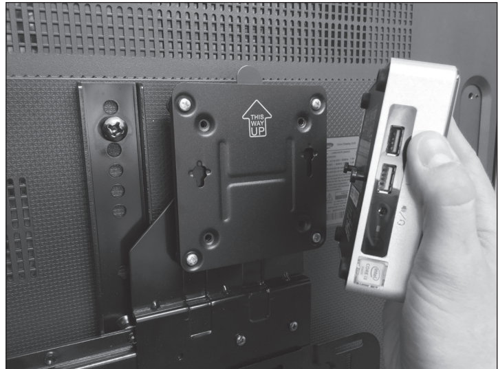
Figure 6: Attaching Screws to Back of the Computer (Left) Attaching Computer to the Computer Mounting Bracket (Right)
