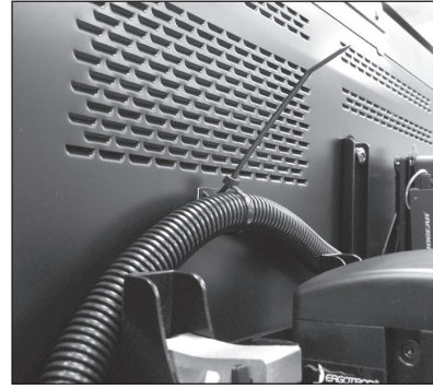
Figure 13: Feeding Zip Tie into Mounting Base (Left), Securing Zip Tie (Right)
